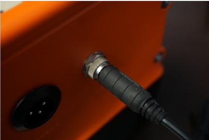
4. Once charger plug is securely fastened to the Pulsator, turn on the machine. The Charge indicator lights will advance through all four, in green. The Power Limit "0" light and Mode "Manual" light will also be lit.
