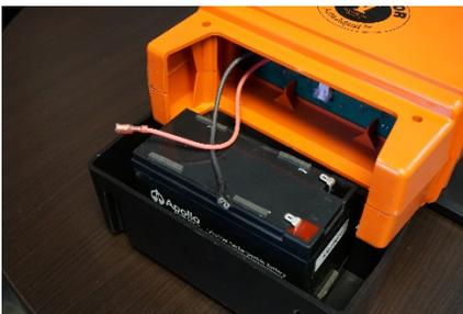
Remove the plastic caps from the battery terminals and attach the cables to the terminals, black to black and red to red.
